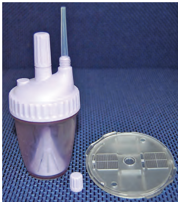
▲ FIGURE 3 Fill-FLOTAC and Mini-FLOTAC apparatus. Image courtesy of Dr. Laura Rinaldi, University of Naples
